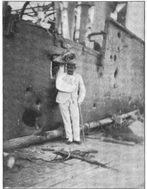
FROM A PHOTOGRAPH TAKEN AT PORT ARTHUR. SUPERSTRUCTURE OF THE "CHEN YUEN," SHOWING DAMAGE.
