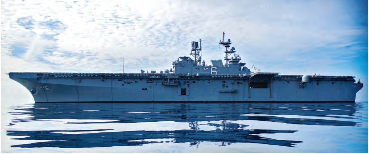
The amphibious assault ship USS America (LHA-6), here off the coast of San Diego, joined the Fleet in October 2014. The first ship of her class and the fourth to bear the name, the America is optimized for aviation and capable of supporting current and future aircraft such as the MV-22 Osprey and F-35B Joint Strike Fighter.
