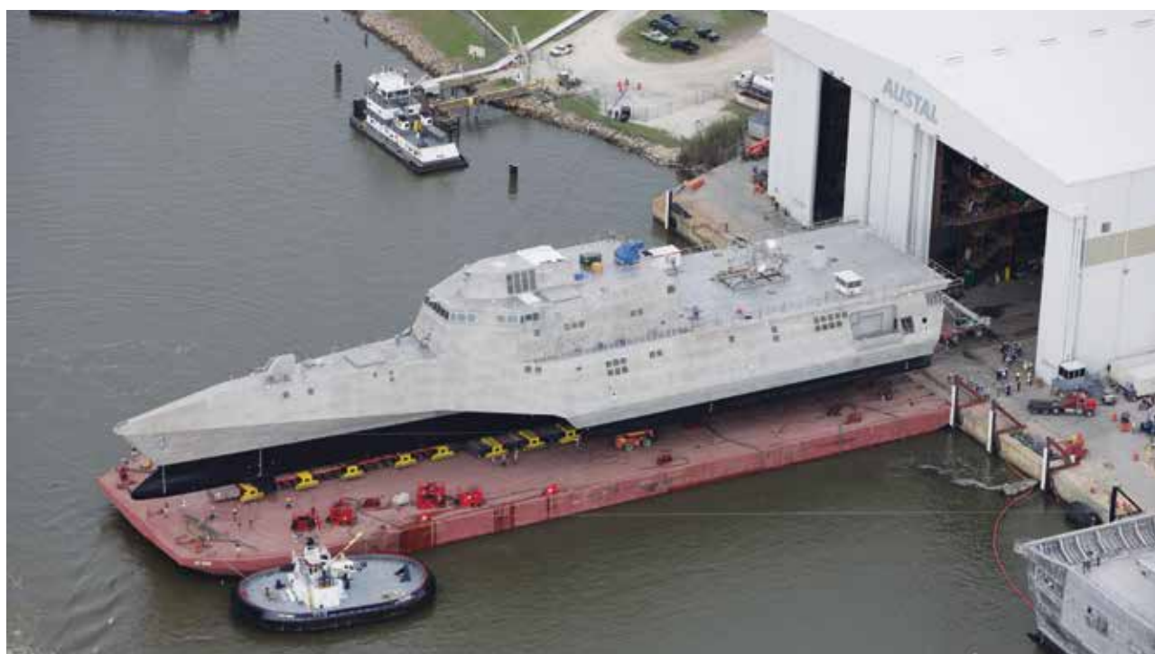
The Navy's newest littoral combat ship, the USS Coronado (LCS-4), shown here in her January 2011 roll-out at the assembly bay of the Austal USA shipyard in Mobile, Alabama, was commissioned on 14 January 2012. The vessel is designed to operate in waters less than 20 feet deep and to speed along at 40 knots. Four more LCSs are under construction or are in pre-production stages.
